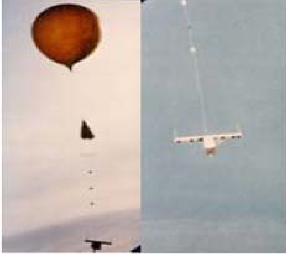
Figure 3: Photograph of a thermosonde (left) and the boom (right) [Adapted from Adair, 2005]
